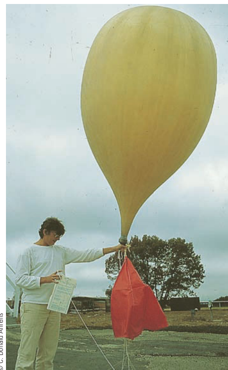
● FIGURE 4 The radiosonde with parachute and balloon.
