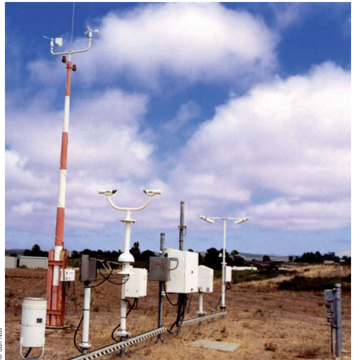
● FIGURE 3.30 The instruments that comprise the ASOS system. The max-min temperature shelter is the middle box.
