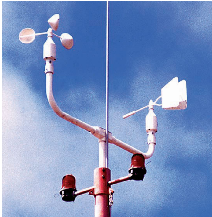
● FIGURE 9.19 A wind vane and a cup anemometer. These instruments are part of the ASOS system. (For a complete picture of the system, see Fig. 3.30, p. 83.)
