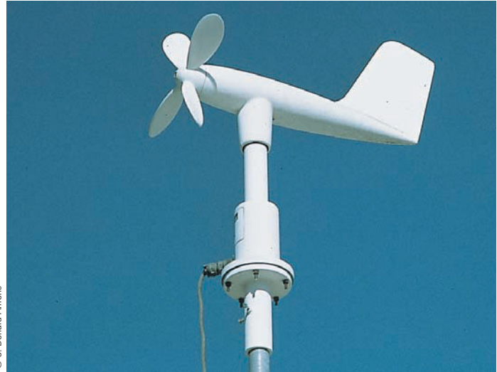
● FIGURE 9.20 The aerovane (skyvane).
