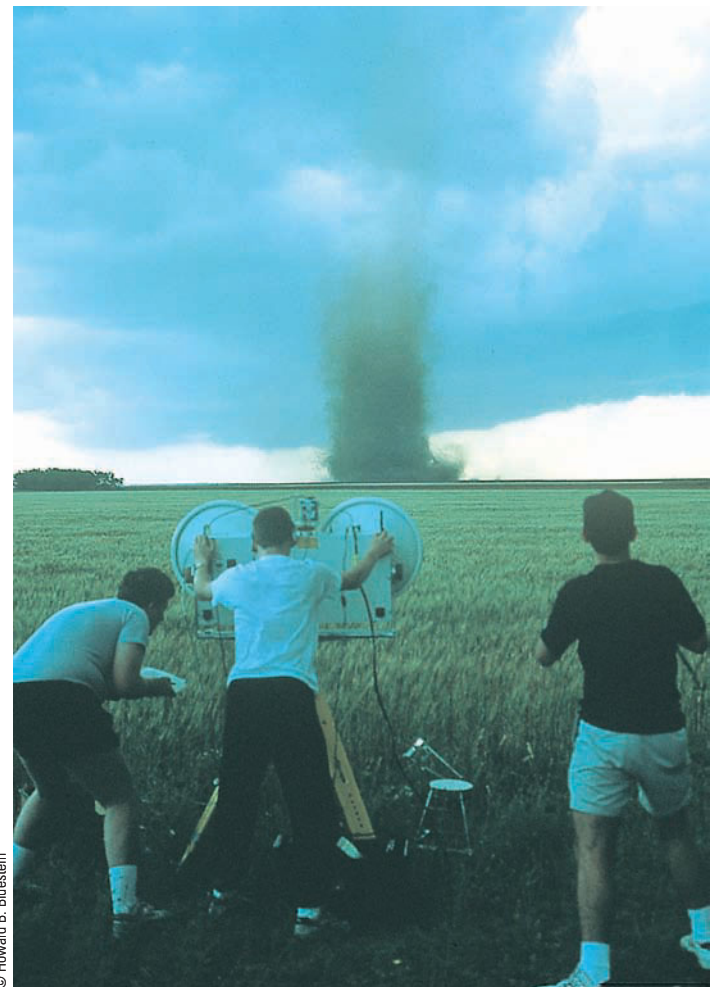
● FIGURE 14.50 Graduate students from the University of Oklahoma use a portable Doppler radar to probe a tornado near Hodges, Oklahoma.
